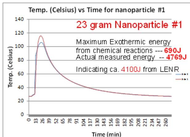
**FIGURE 3.** Temperature profile during the 60 psi deuterium loading of the #1 nanoparticles. Two different curves were recorded by two thermocouples attached to the sample cylinder at different sites. In this case, 99.99% deuterium gas was used.
