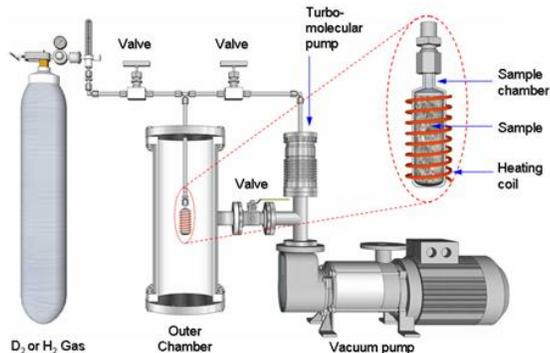
FIGURE 2. Schematic of the gas-loading system.
