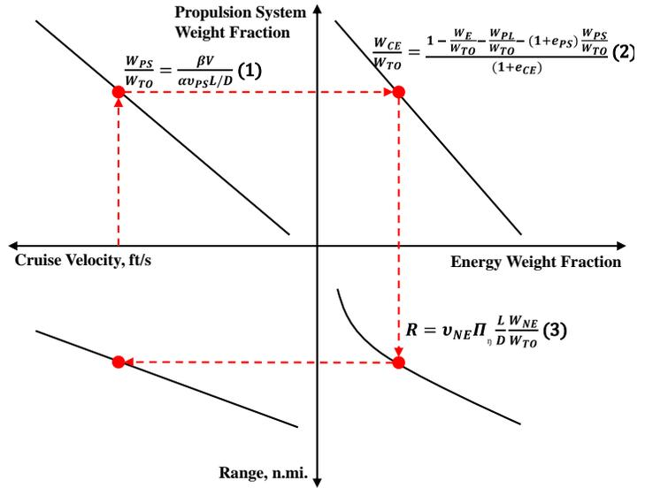
Figure 5. NAM ratio diagram plotting process<sup>14</sup>
