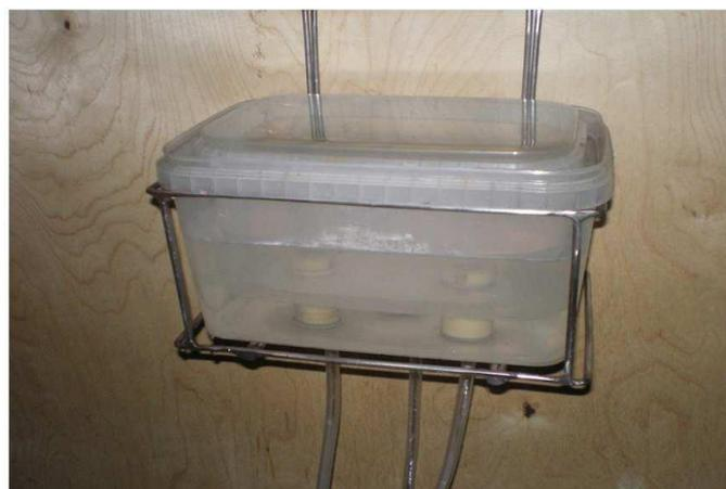
Figure 4: Water flow rate damping tank
